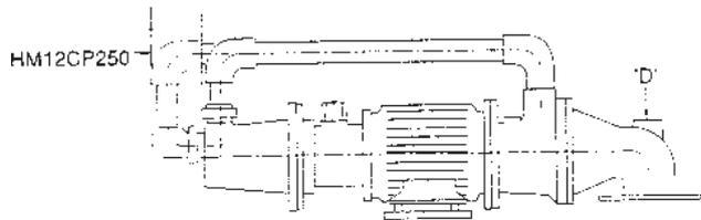
Time can be saved by fitting a reliable vacuum gauge to the pump priming connection on the suction side as in the event of restriction this will immediately be revealed by a reading well in excess of approximately 3" HG (76mm HG) which can be taken as an average figure for normal use in conjunction with a fibreglass tank.
